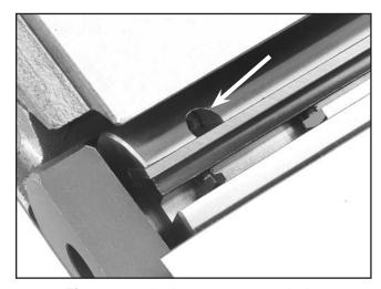
Figure 44. Jack screw access hole.
